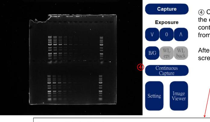
(4) Continuous Capture is the exposure value that can continuously shoot screens from -2 to +2.
