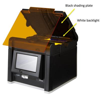
To shoot fluorescent film images, please slide the black shading plate (with the flannel side outwards) into the rail to cover the white backlight plate of the upper cover to avoid reflections.
